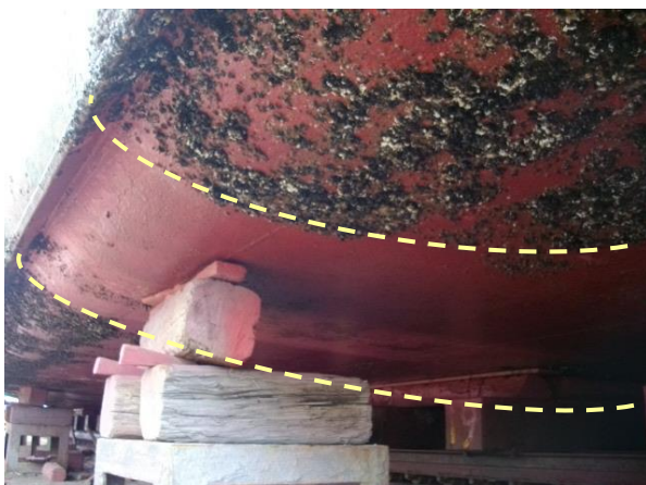
1 year performance after long anchorage in Tokyo Bay
